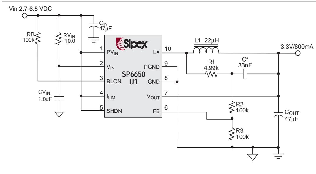
Figure 16. Additional Application Circuit with Low Output Ripple
