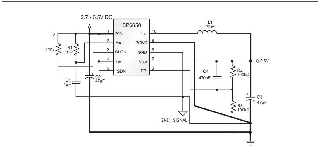
Figure 21. Application circuit with highlighted power traces.
